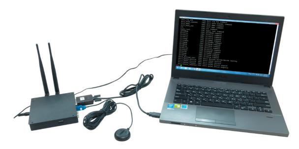
2. Painless enable V2X on existing outdoor Wi-Fi AP: Directly connect OBU-201U to existing Wi-Fi AP through Ethernet port. Deploy V2X application software on Linux through OSLink and TCP/IP.
