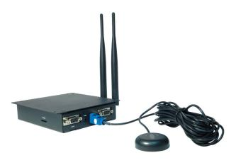
The OBU-201U is a standalone V2X on-board-unit containing 3-CPU core processor, dual channel DSRC RF transceiver, GNSS receiver, and hardware security with embedded IEEE 1609.x protocol stacks running on ThreadX RTOS. Companies can directly deploy V2X application programs on OBU-201U internal system through SDK and protocol stack API.
